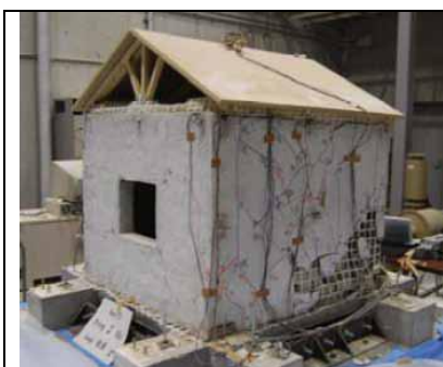
Figure 4-14 Full scale adobe model reinforced with pp band after a shake table test
